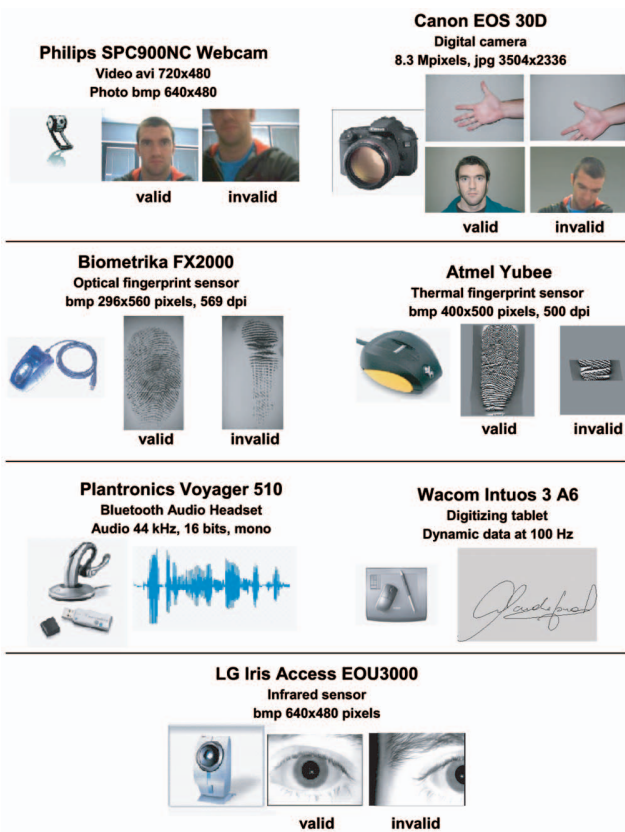
Fig. 3. Hardware devices used in the acquisition of DS2 together with acquisition samples.
