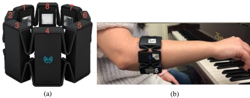
Fig. 1. (a) The Myo armband showing 8 channels of EMG electrodes. (b) A photo of the standardized placement of the Myo armband when collecting raw IMU and EMG data.
