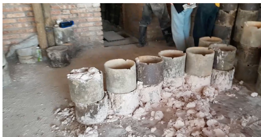
Photograph 12: (Clockwise from top left): Labourers preparing rare earth sediment for burning; Transferring rare earth sediment to clay pots and into the wood-fired furnaces; Clay pots with rare earth sediment waiting to be burnt. Chipwe/Pangwa, 2023.
