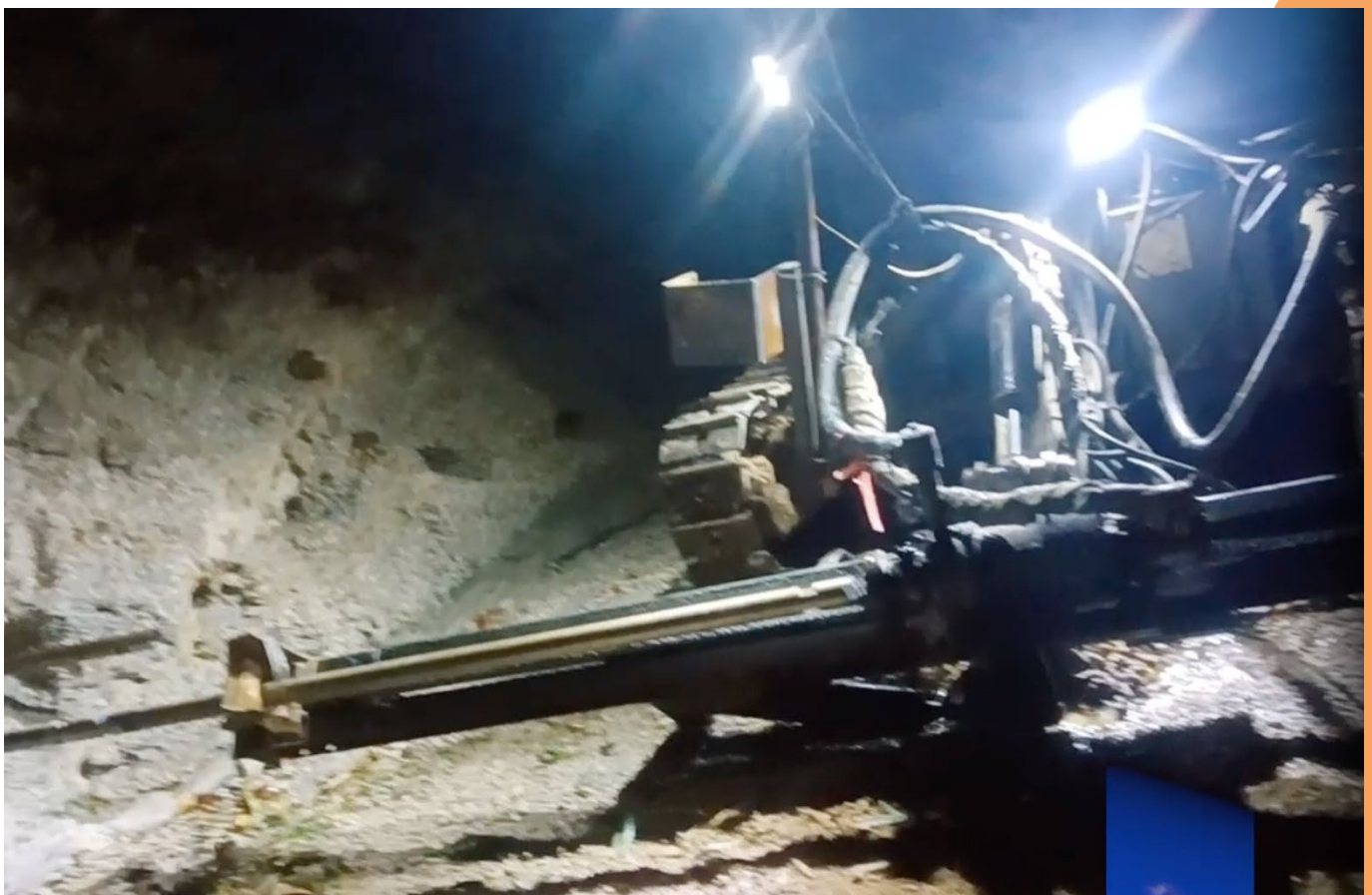
Photograph 2: Drilling pipes into the hillside. Some mining work takes place around the clock with workers divided into day and night shifts
