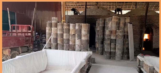
Photograph 11: Rare earth sediment being prepared for burning in the furnaces. Chipwe/Pangwa, 2023.
