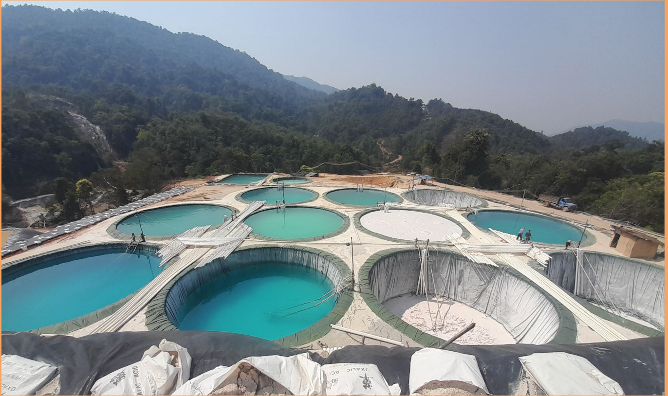
Photograph 10: Workers prepare to dig out the rare earth sediment from collection pools. Chipwe/Pangwa, 2023.
