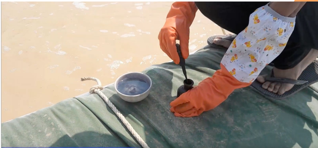
Photograph 9: A worker tests the leachate in the collection pools to measure the concentrate of rare earths. Chipwe/Pangwa, 2023.
