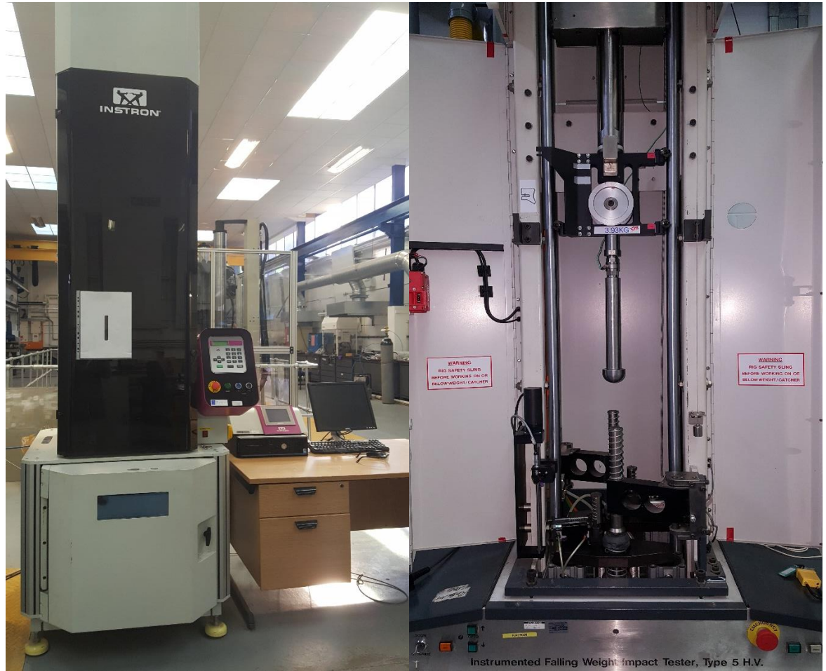
Figure 15: (on the left) initial impact tower, (on the right) impact tower used for the tests
