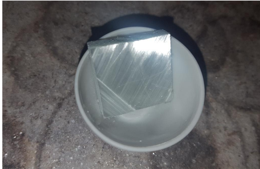
Figure 32: Specimen after resin- burn off test
