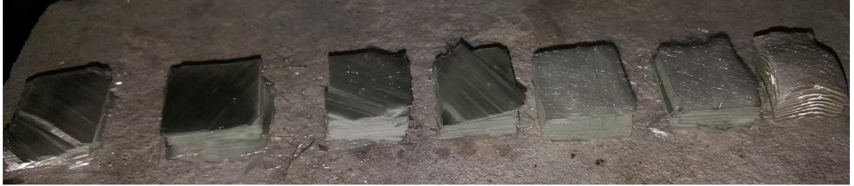
Figure 33: Burned specimens (6000C) of the parametric study used to identify the optimal burn time
