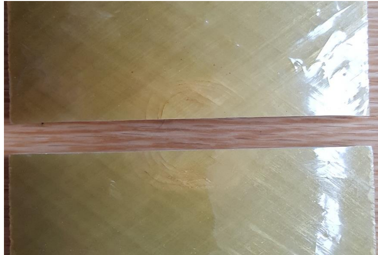
Figure 38: Impacted specimen cut in the middle with a diamond cutter
