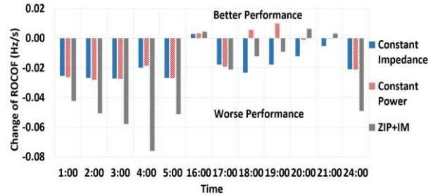
Figure 8. Mean Value of Absolute Change of ROCOF with Different Load Models in Case 3 (60% Renewable and 60% Loading)
