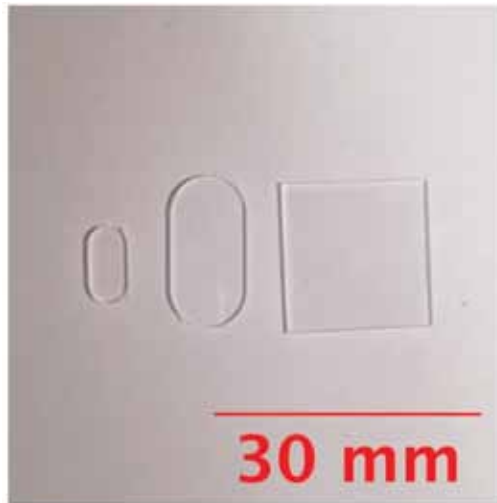
FIGURE 14 Photograph showing examples of 1.0 mm thick quartz sheet cut to round corners with radii of 2 and 4 mm and a right angle square structure cut with a side length of 16 mm.
