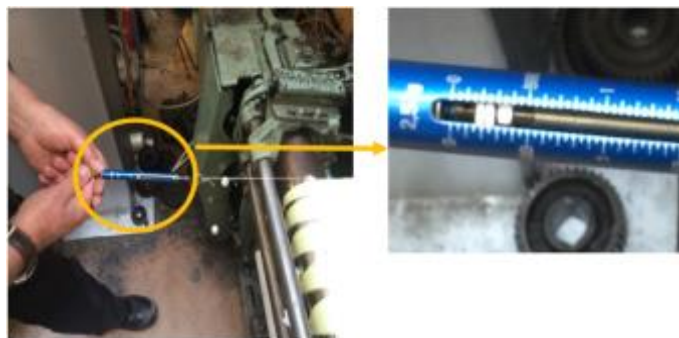
Figure 3-7 Spring tension metre measures the tension of yarn
