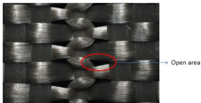
Figure 3-17 Leno line under microscope
