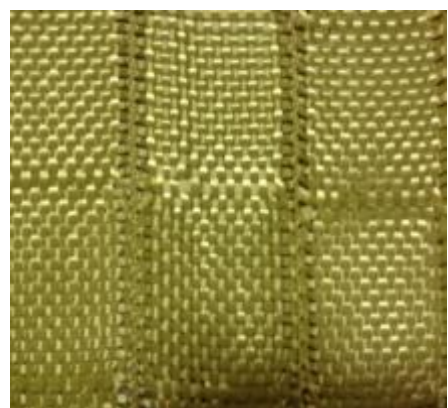
(f) Leno and double-pick insertion
