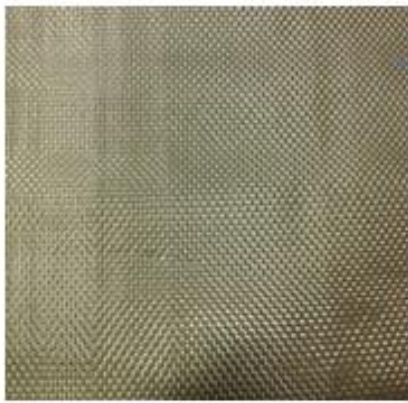
(c) Plain fabric with cramming insertion
