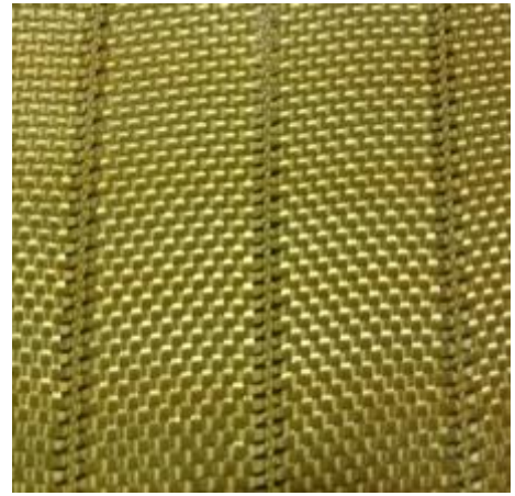
(b) Plain fabric with leno insertion
