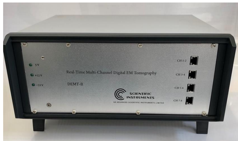
Figure 4.6 The picture of the custom designed EM inspection instrument.
