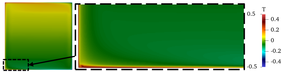
522 Fig. 15. An instantaneous snapshot of the RANS temperature from a hybrid simulation in which the LES zone 523 weight was calculated using Equation (44). A zoomed-in view of the contours near the bottom left corner is 524 provided as well.
