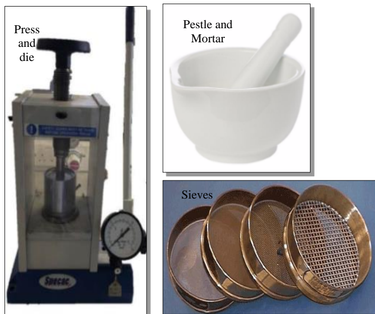
Figure 2-3 Catalyst preparation using press, die, mortar and pestle, and molecular sieves.
