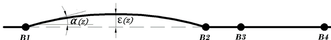
Figure 7. Schematic of deflection assumed at shaft 1, Sh1, in shaft bow simulation.
