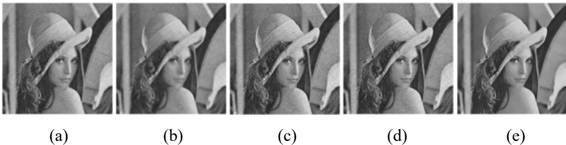
Figure 2.1: An illustration of image denoising [152]: (a) Wiener filtering [153], (b) Bilateral filtering [154], (c) PCA method [155], (d) Wavelet transform domain method [156], (e) BM3D [157].
