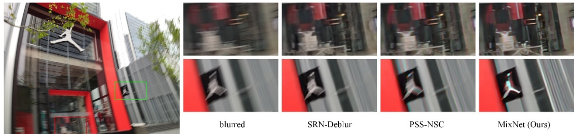
Figure 3.11: Testing results of the proposed MixNet for image deblurring on RWBI dataset.
