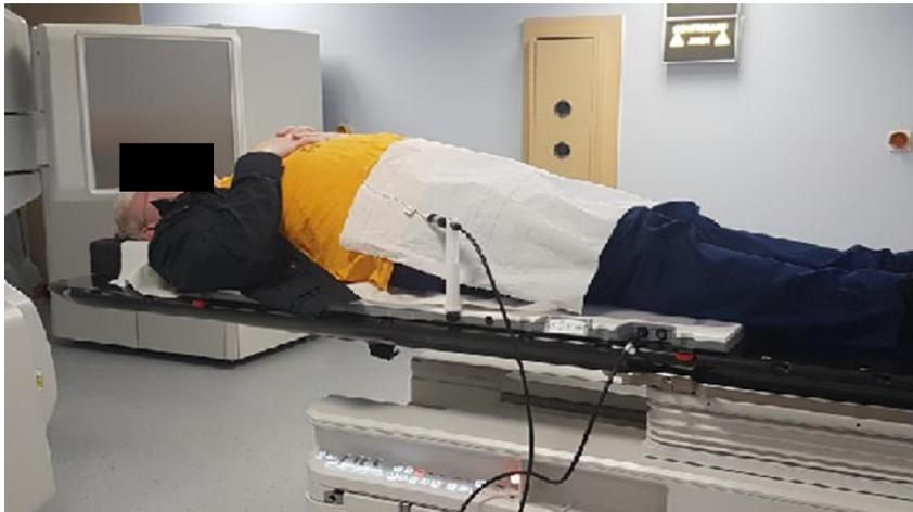
**Fig B1:** Image of the set up for the RayPilot system on a linac. The patient is positioned on the couchtop sensor plate which is connected by cable to the transmitter.
