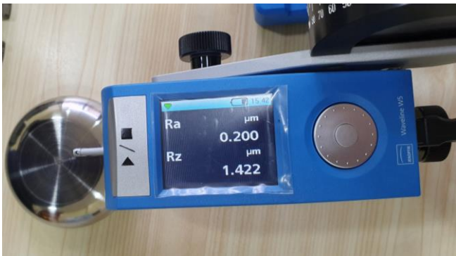
Figure 2. Surface roughness measurement of a polished electrode surface.
