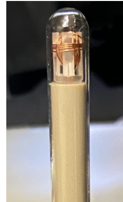
Fig. 9. Tip of the B-dot probe showing the three coils.
