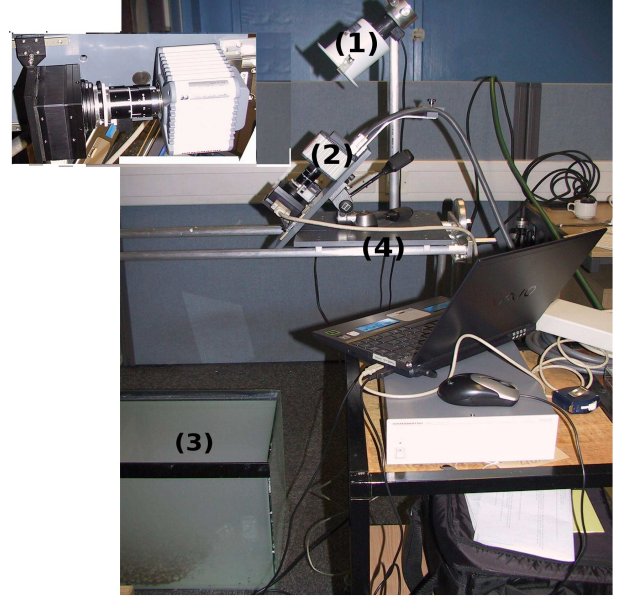
Fig. 1. Water tank experimental setup. 1)Light source 2)Multispectral camera 3)Water tank 4)Translation stage.
