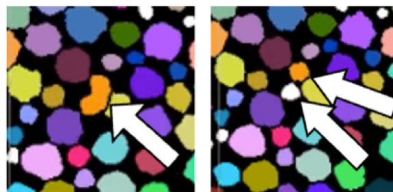
Fig. 5. Fibril branch point. The orange fibril branches to become two separate fibrils. The algorithm currently records them as two separate fibrils and does not record the branching. (For interpretation of the references to colour in this figure legend, the reader is referred to the web version of this article.)
