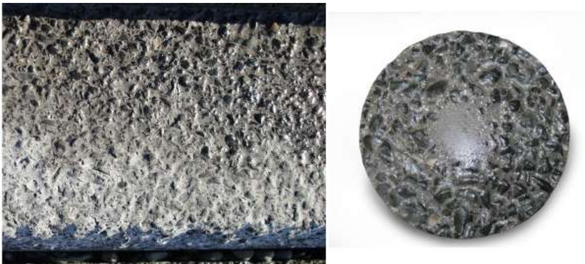
Figure 2: Abrasion pattern on 375mm tread of stepped revetment at reference site (left) and on test sample no.1 after 72 hours (right)
