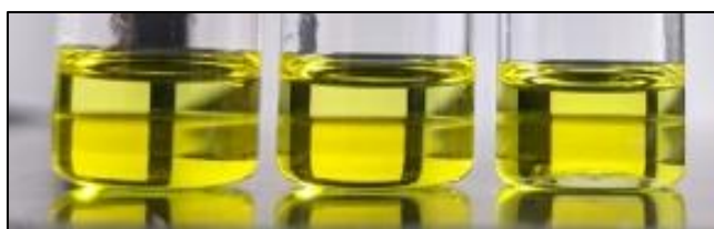
Figure 43. Third phase observed for organic phase with extraction conditions of 6 M HNO 3 , U 180 g.L -1 T = 293 K. Photographed at ambient conditions. Clear boundary can be seen between top, lighter layer and heavy bottom phase. T = 293 K
