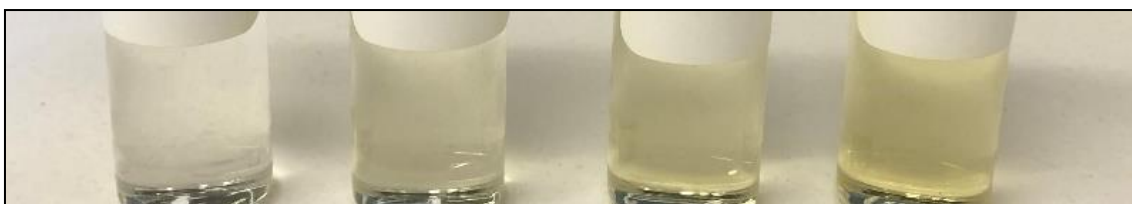
Figure 65. Samples of 0.2 M TODGA + 0.5 M DMDOHEMA in n-dodecane uncontacted after undergoing \gamma -radiolysis with respective total doses (left to right) of 0, 250, 500, 750 kGy irradiation
