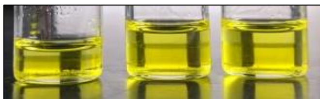
Figure 43. Third phase observed for organic phase with extraction conditions of 6 M HNO 3 , U 180 g.L -1 T = 293 K. Photographed at ambient conditions. Clear boundary can be seen between top, lighter layer and heavy bottom phase. T = 293 K
