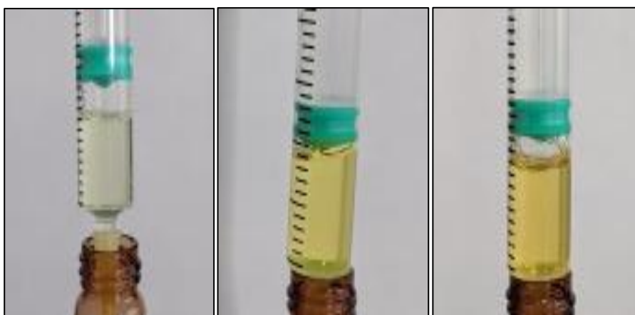
Figure 64. Samples of 1 M DEHiBA in n -dodecane (pre-contacted with 4 M \text{HNO}_3 ) after undergoing \gamma -radiolysis with respective total doses (left to right) of 250, 500, 750 kGy irradiation
