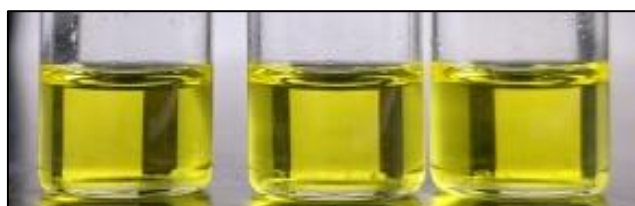
Figure 44. Third phase observed for organic phase with extraction conditions of 6 M HNO 3 , U 180 g.L -1 T = 313 K only when brought to 293 K. Photographed at ambient conditions. Boundary can be seen between top, lighter layer and heavy bottom phase.
