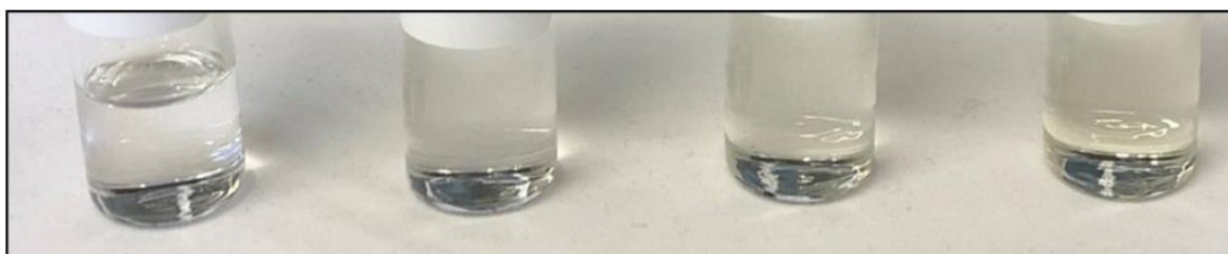
Figure 63. Samples of 1 M DEHiBA in n -dodecane (uncontacted) after undergoing \gamma -radiolysis with respective total doses (left to right) of 0, 250, 500, 750 kGy irradiation
