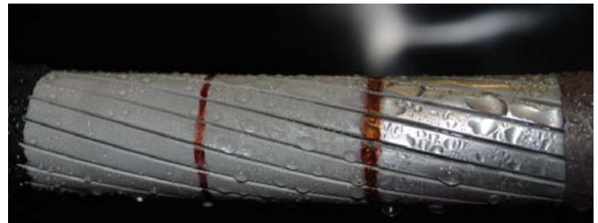
Fig. 3. Formation of water droplets on the surface of different hydrophobicities
