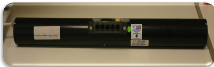
Figure 2.1 TL20W/12 UVR source. Hand held broadband UVB light source with five graduated filter apertures allowing a series of UVR doses to be administered simultaneously.
