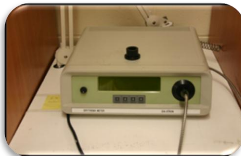
2. 7 Reflectance instrument used to measure erythema index
