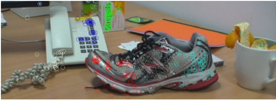
Fig. 5. The set of clustered features in a scene input image. The advantages of spatial clustering are clearer here as various objects have are roughly separated by the different clusters so as to provide more information when matching features.
