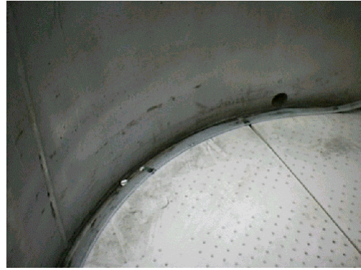
Figure 4.17: Filter cloth & support plate
