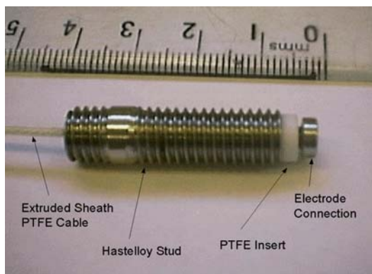
Figure 6.39: Mk2 stud assembly
