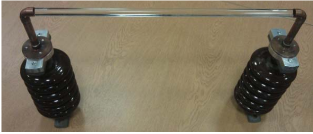
Figure 4. Glass rod conductivity measurement system
