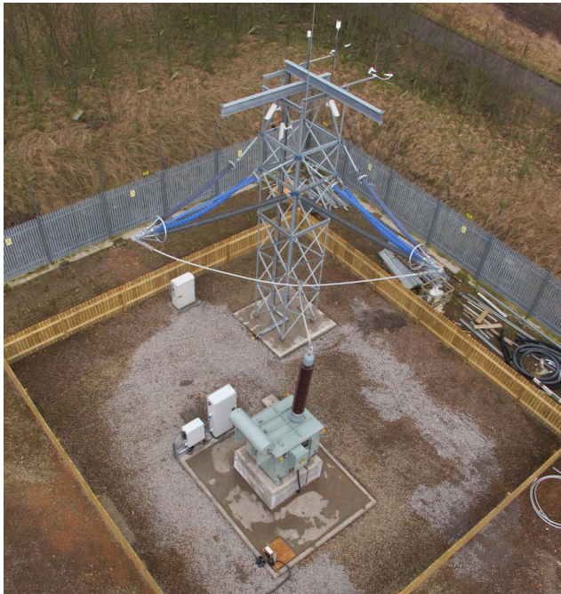
Figure 2. Trial site overview. The reference cross-arms consist of a range of insulator designs
