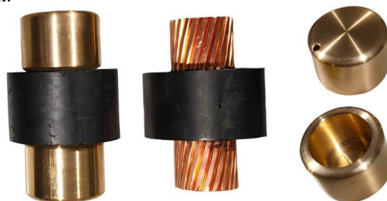
Figure 1. Offcuts of 66 kV XLPE cable were prepared into shorter-length samples for laboratory testing and the brass end-cap design is to minimise electrical noise.
