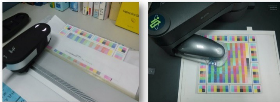
Figure 6. Measure the puzzle-like test target using an X-rite i1 spectrophotometer in either manual way (left) or automatic way (right). Note that the inverse side also contains the same number of colour patches.
