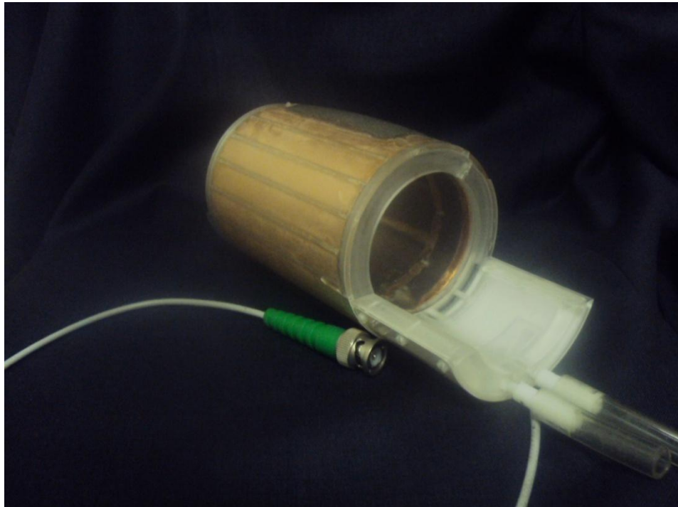
Figure 4.1: The 8cm internal diameter volume coil. The full animal was positioned within the coil ( cf. the Surface coil - Figure 3.2)
