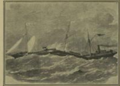
THE "CONNECTOR," A JOINTED IRON STEAM-SHIP, 1885. The "Connector" was tried in the Thames in July 1885. She proved herself thoroughly seaworthy in heavy weather. All the masts are joggled slightly, and it was thought that there should be a similar arrangement on the deck.
