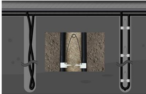
Figure 7.4: Typical vertical heat exchanger installation on the left, compared to a GEOCLIP installation on the right ( www.geoclip.com ).
