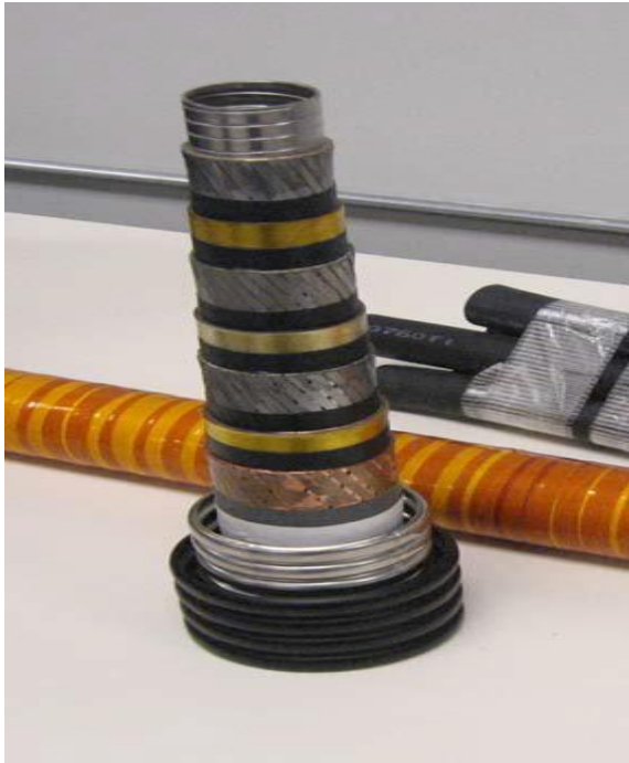
Figure 10: Showing the Triaxial design with “nitrogen impregnated, cold insulation between layers” [18]
