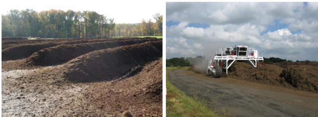
Figure 3 Composting method in windrows (Adapted from EPA, 2002)
