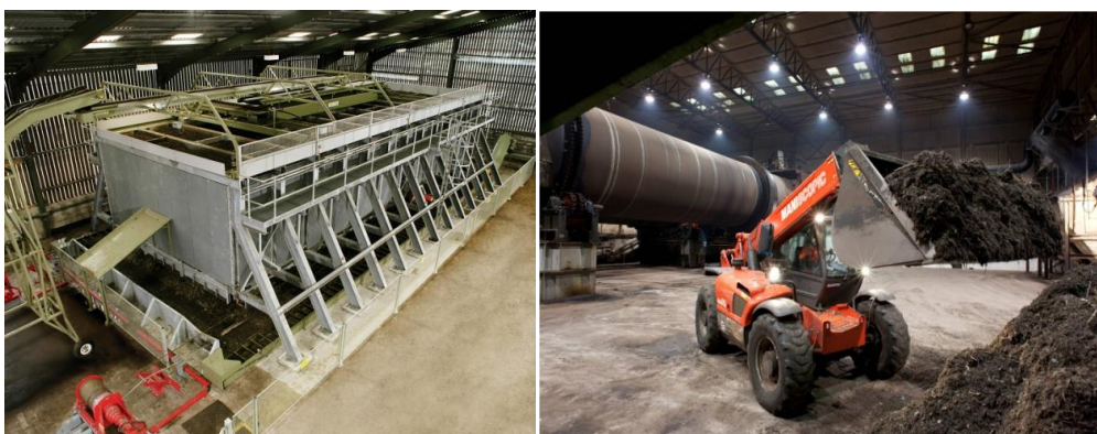
Figure 4 In-vessel composting method (Adapted from EPA, 2002)
