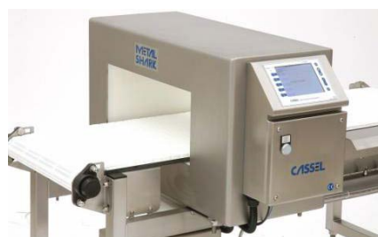
(b) Metal detector for meat products (Cassel Messtechnik, 2017)
