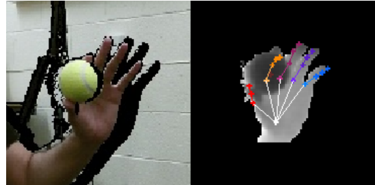
Fig. 1: We present a new two stage discriminative system for estimating the joint and object locations of the hand interacting with an object from the depth image. In this image, the index finger is almost completely occluded by the ball.
