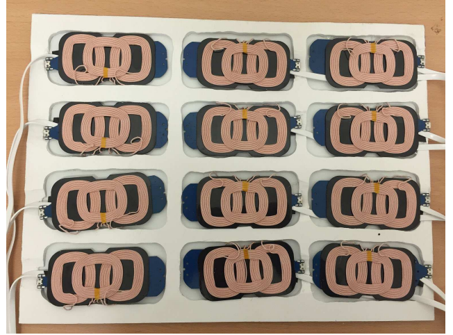
Fig. 5 The utilised prototype charging pad ( 30 \times 40 cm 2 ) including 12 independent cells ( M_{4,3} ) supplied with a USB hub (5 V, 1 A).
