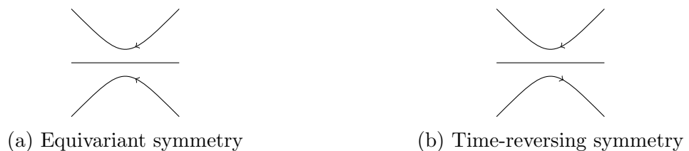
Figure 2.1: Phase portraits of planar flows that are symmetric with respect to a horizontal reflection. In (a) the reflection is an equivariant symmetry and in (b) the reflection is a reversing symmetry.
