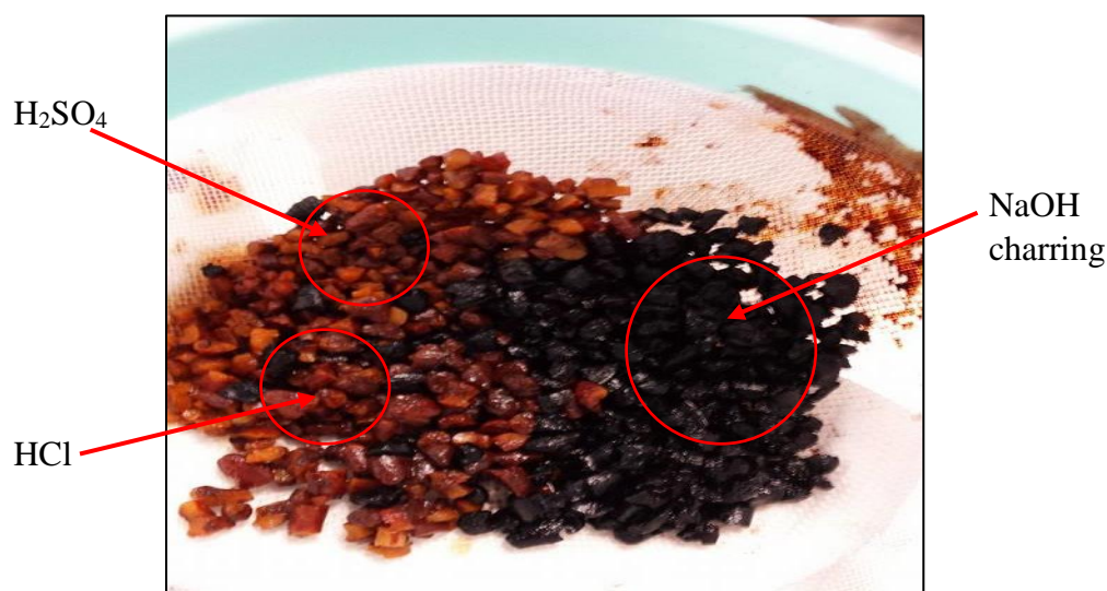
Figure 5.4. Effect of various types of solvents, H 2 SO 4 , HCl and NaOH, on date seeds after hydrolysis using (5:1v/w) ratio and 100 °C.
