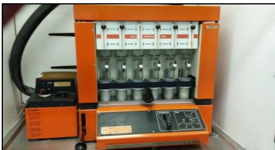
Figure 4.4. A Soxtec system HT 1043 extraction unit (Velp Scientifica, Europe) equipped with six thimbles.
