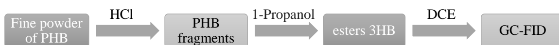
Figure 4.3. Schematic diagram for PHB extraction from C. necator cells using Riis, and Mai et al., method.
