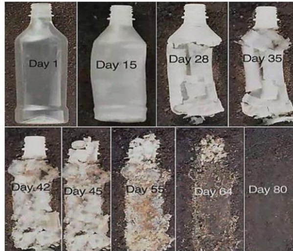
Figure 2.4. PHA bottle biodegradation, type BiopolTM, by incubation in mud for 80 days (Sudesh et al., 2000).
