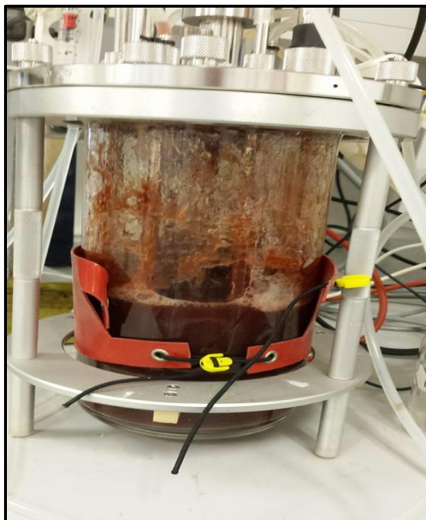
Figure 4.5. Autoclavable benchtop laboratory bioreactor utilised for fermentation and cell culture
