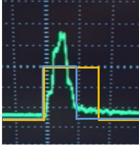
FIGURE 6.3: Pulse shape used during the francium experiment. The green line is the signal read on a photodiode placed after the setup. The blue and orange lines are the signals being supplied to the two Belkhe switches. The pulse widths of the switching signals were 100 ns and 170 ns. Each horizontal division is equivalent to 100 ns.
