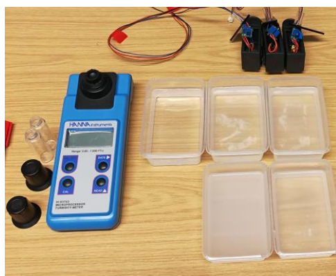
Fig. 3. Prepared solution as water samples, the concentration of fat particulates within each sample is changed by mixing the particles with distilled water. HI 93703, as a reference meter, is used to determine the turbidity of each sample.
