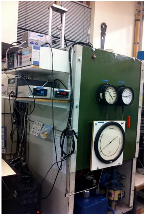
Figure 3.13 Picture and Schematic diagram of seismic velocity rig
