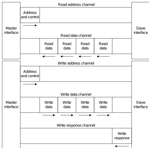
FIGURE 2 Channels in AXI interface, taken from [26].
