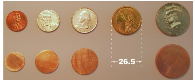
Fig. 5. Subset of US coins and copper disks used for tensor measurements. Scale in mm. Top row (left to right); cent, nickel, quarter dollar, dollar and half dollar. Bottom row; validation disks in the sizes of the dime, nickel, quarter dollar and half dollar.
