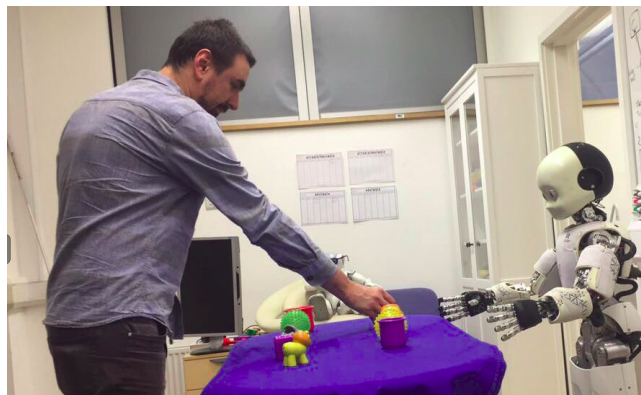
Fig. 1: The iCub learns new vocabulary through the use of complementary gesture-speech combinations.
